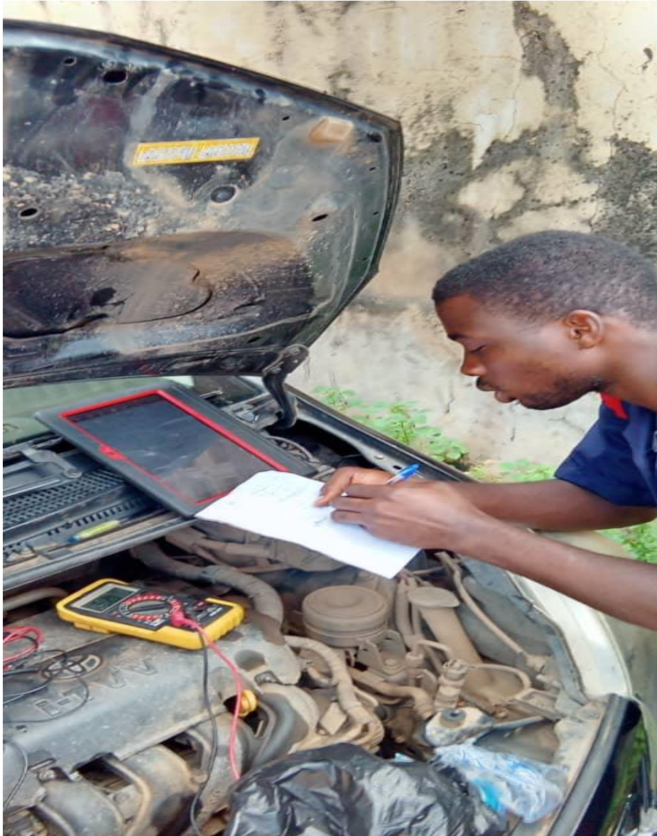
Figure.3 6 Calibrating CTS Sensor
