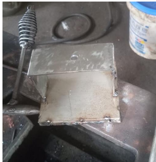
Figure 3.13: Fabrication of the Stamping Base of the Toggle Clamp
