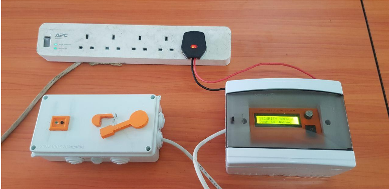
Fig (Door sensor detecting security breach)
